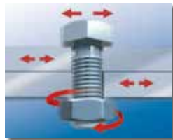
Vibration and loosening.
